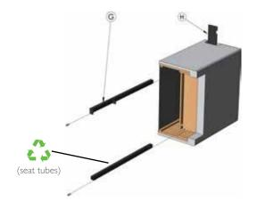
**G & H:** Using the Philips screwdriver, remove the screw securing the seat tubes to the seat box and slide them out. Next slide out the seat box support rail.
