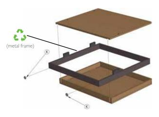
J: As you did with the seat and back boxes, carefully remove the fabric and foam from each arm box. Next taking the flat blade screwdriver and hammer, pry away one side of the arm box. Remove the metal frame from the box. Now remove the glides using the flat blade screwdriver and hammer:
