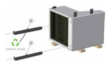
D: If you are disassembling a single chair, it may be easier now to place blocks of wood under the chair so that the seat and back support rails clear the floor. Using the Philips screwdriver, remove the screws from the retainer straps securing the support rails in place. It may require a screwdriver and a hammer to remove the straps, particularly with a 2 or 3 seat arrangement as there will be some binding on the rails if the seat boxes are resting on the floor.
